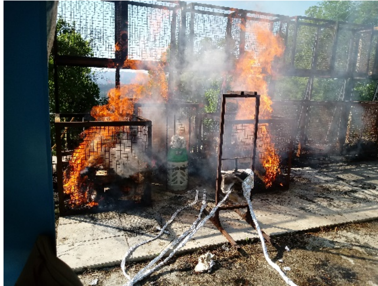
Figure 5: Composite canister test
